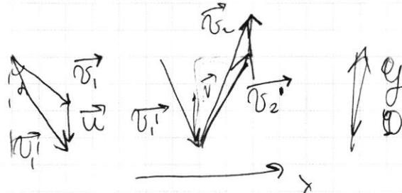
$$v_1 \sin \alpha = v_2 \sin \beta$$
