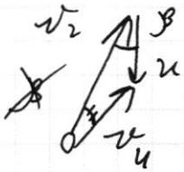
$$v_4^2 = v_2^2 + u^2 - 2uv_2 \cos \beta$$
