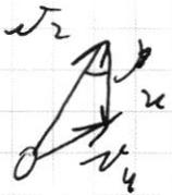
$$v_4^2 = v_2^2 + u^2 - 2uv_2 \cos \beta$$
