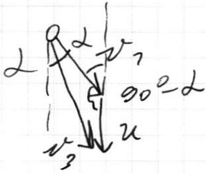
$$v_3^2 = v_1^2 + u^2 - 2v_1u \cdot \cos(90^\circ - \alpha) \quad \text{'' Синус}$$
