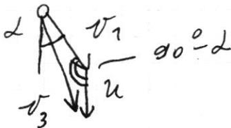
$$v_3^2 = v_1^2 + u^2 - 2v_1 u \cos(90^\circ - \alpha)$$
