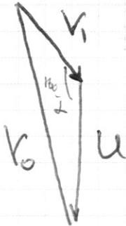
$$v_0 = \sqrt{v_1^2 + u^2 + 2v_1u \cos \alpha}$$
