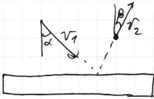
$$v_2 \sin \beta = v_1 \sin \alpha \Rightarrow$$
