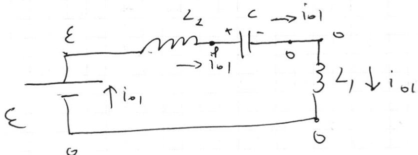
$$\left. \begin{aligned} E - \ell &= L_2 \frac{\Delta i}{\Delta t} = \frac{L_2 i_{01}}{\Delta t} \\ i_{01} &= C \frac{\Delta V}{\Delta t} = \frac{C(\ell - 0)}{\Delta t} \end{aligned} \right\} \Rightarrow \Delta t = \frac{L_2 i_{01}}{E - \ell} \Rightarrow \frac{L_2 i_{01}}{E - \ell} = \frac{C \ell}{i_{01}}$$
