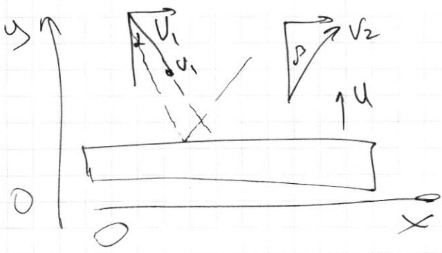
$$v_1 \sin \alpha = v_2 \sin \beta$$
