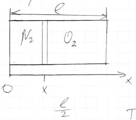
$$\begin{aligned} pSx &= JR T_{N_2} \\ pS(l-x) &= JR T_{O_2} \\ pS(2x-l) &= JR(T_{O_2} - T_{N_2}) \\ 2pSdx &= 2JRdT \\ pSdx &= JRdT \end{aligned}$$
