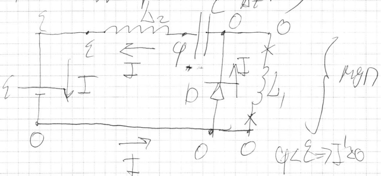
$$E - \phi = L_2 \frac{\Delta I}{\Delta t} \quad \phi = E = L_2 I'$$
