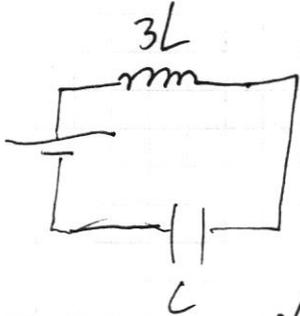
$$T_2 = 2\pi\sqrt{3LC}; \quad T = T_1 + T_2 = \pi\sqrt{3LC} + \pi\sqrt{7LC}$$
