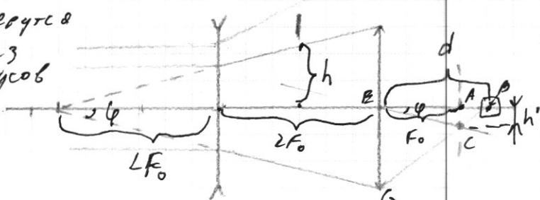
$$\sin \varphi = \frac{\vartheta}{2} : 4F_0 = \frac{\vartheta}{8F_0} \quad \text{так } \triangle ABC \sim \triangle BEG$$
