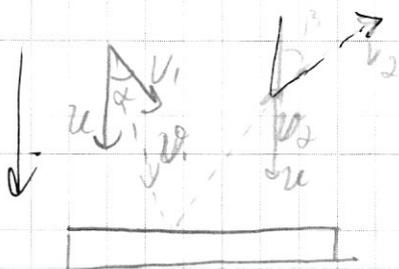
$$v_1^2 = (v_1 \cdot \cos \alpha + u)^2 + (v_1 \cdot \sin \alpha)^2$$
