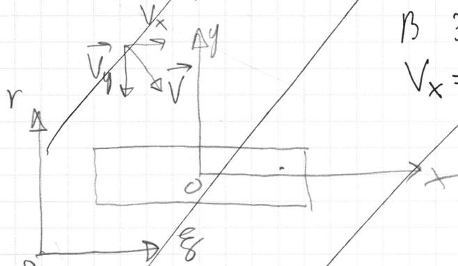
$$V_x = V_1 \sin \theta; V_y = [V_1 \cos \theta + U]$$
