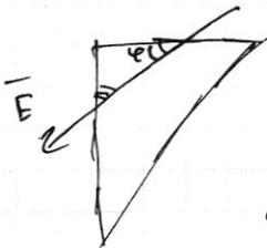
$$S E \sin \varphi = \frac{SS}{\epsilon_0} = S E \cos \varphi = \text{for } \varphi = 45^\circ$$
