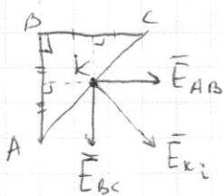
$$\vec{E}_{BC} + \vec{E}_{AB} = \vec{E}_{K_1}; |E_{K_1}| = \sqrt{E_{BC}^2 + E_{AB}^2} = E_{BC}\sqrt{2} -$$
