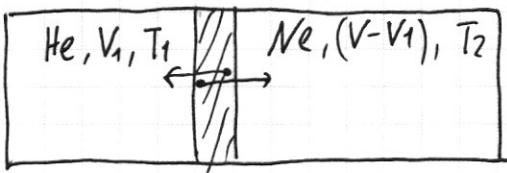
$$1) PV_1 = \cancel{P}RT_1 \rightarrow \frac{V_1}{V_2} = \frac{T_1}{T_2} = \frac{3}{4}$$
