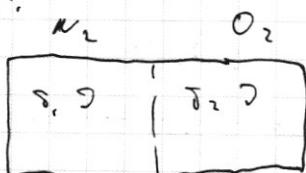
$$p_0 V_{10} = DRT_1, \quad p_0 V_{20} = DRT_2 \Rightarrow \frac{V_{10}}{V_{20}} = \frac{300}{500} = \frac{3}{5}$$
