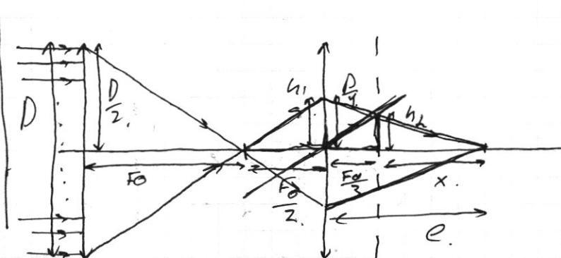
$$a) \left\{ \begin{array}{l} \frac{h_1}{\frac{D}{2}} = \frac{\frac{F_0}{2}}{F_0} \Rightarrow h_1 = \cancel{\frac{D}{2}} \frac{F_0}{4}. \end{array} \right.$$
