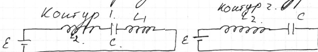
$$\left\{ \begin{array}{l} q = CU \\ U = E - E_1 - E_2 \\ E_1 = L_1 \cdot \dot{q} \\ E_2 = L_2 \cdot \dot{q} \\ \Rightarrow \omega = \frac{1}{CL_1 + L_2} \end{array} \right. \Rightarrow \tau_1 = 2\pi \sqrt{C(L_1 + L_2)}$$
