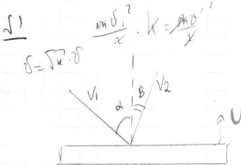
$$\begin{cases} (k \cos \alpha + U) \cdot k + U = V_2 \cdot \cos \beta \\ V_1 \cdot \sin \alpha = V_2 \cdot \sin \beta \Rightarrow V_2 = V_1 \cdot \frac{\sin \alpha}{\sin \beta} \end{cases}$$
