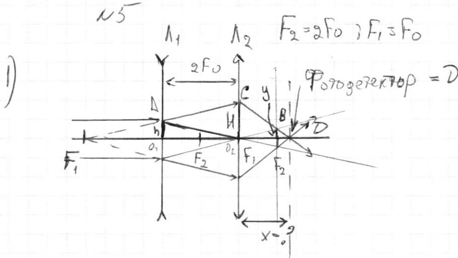
$$\frac{h}{2F_0} = \frac{y}{F_0} \quad \triangle O_1 O_2 A \sim \triangle O_2 F_2 B$$
