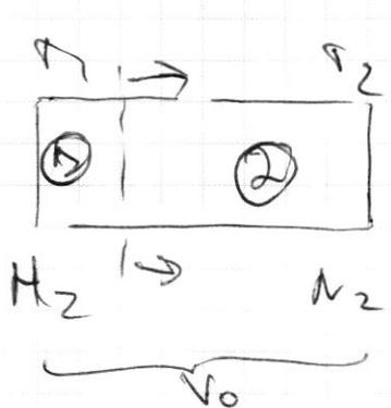
$$\Delta) p(H_2) = \frac{\nu R T_1}{V_1} = p(N_2) = \frac{\nu R T_2}{V_2}$$
