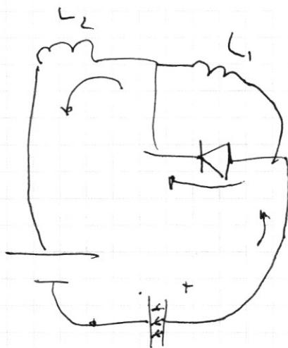
$$\begin{aligned} E &= L_2 \dot{i} + L_1 i + \frac{q}{C} \\ E &= (L_2 + L_1) \ddot{i} + \frac{q}{C} \\ E &= 3L \ddot{i} + \frac{q}{C} \\ \ddot{i} + \frac{q}{3LC} - \frac{E}{3L} &= 0 \end{aligned}$$
