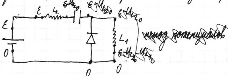
$$\begin{aligned} \dot{I}_{L_{10}} &= 0 \\ \dot{I}_{L_{20}} &= 0, \quad W_0 = \frac{L_1 I_{10}^2}{2} + \frac{L_2 I_{20}^2}{2} + \frac{C U_0^2}{2} = 0 \\ U_{C0} &= 0 \end{aligned}$$
