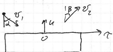
$$P_T = m v_1 \sin \theta = m v_2 \sin \beta$$
