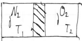
$$1) \begin{cases} p_1 V_1 = \nu R T_1 \\ p_2 V_2 = \nu R T_2 \end{cases} \Rightarrow \frac{V_1}{V_2} = \frac{T_1}{T_2} = \frac{3}{5}$$
