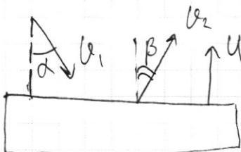
$$1) v_1 \sin \alpha = v_2 \sin \beta$$
