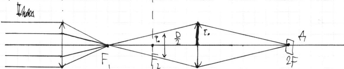
$$S_{\text{img.}} = \frac{1}{4} S_{\text{object.}} = \frac{1}{4} \cdot \frac{\pi}{4} \cdot \frac{D^2}{4} = \frac{\pi D^2}{64}$$
