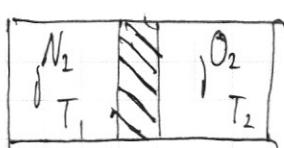
$$1) \begin{cases} p_1 V_1 = \sqrt{RT_1} \\ p_2 V_2 = \sqrt{RT_2} \end{cases} \Rightarrow \frac{V_1}{V_2} = \frac{T_1}{T_2} = \frac{3}{5}$$
