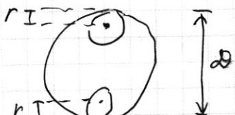
$$t_1 - t_0 = \frac{\varnothing - 2r}{V}$$
