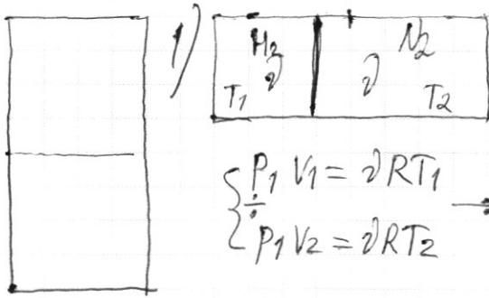
$$\begin{cases} P_1 V_1 = \vartheta R T_1 \\ P_1 V_2 = \vartheta R T_2 \end{cases} \rightarrow \frac{V_1}{V_2} = \frac{T_1}{T_2} = \frac{350}{550} = \frac{7}{11}$$
