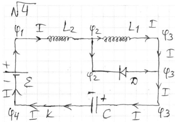
$$\begin{cases} \varphi_1 - \varphi_4 = \mathcal{E} \\ \varphi_1 - \varphi_2 = L_2 \frac{dI}{dt} \\ + \\ \varphi_2 - \varphi_3 = L_1 \frac{dI}{dt} \\ \varphi_3 - \varphi_4 = \frac{q}{C} \end{cases} \Rightarrow \begin{cases} \varphi_1 - \varphi_4 = \mathcal{E} \\ \varphi_1 - \varphi_3 = (L_1 + L_2) \frac{dI}{dt} \\ + \\ \varphi_3 - \varphi_4 = \frac{q}{C} \end{cases}$$
