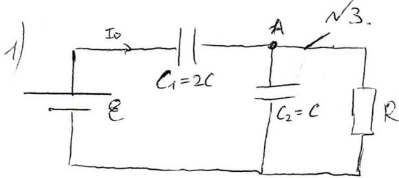
$$C_{\text{общ.}} = \frac{C_1 \cdot C_2}{C_1 + C_2} = \frac{2}{3} C \Rightarrow q = \epsilon \cdot C_{\text{общ.}} = \frac{2C\epsilon}{3}$$
